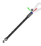
The cord is inextensible. Its effective length can change only if a source of a cord is provided—for example, in the form of a spool. If the second terminus of the cord is another tip, the length of the cord is fixed, and so must be the distance around the pulleys from one tip to the other. This distance is monitored during simulation, through calculations based on the placement and geometry of the pulleys. The two measures—the length and the distance—must always agree.
