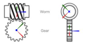
The block represents only the kinematic constraint characteristic to a worm-and-gear system. Gear inertia and geometry are solid properties that you must specify using Solid blocks. The gear constraint model is ideal. Backlash and gear losses due to Coulomb and
