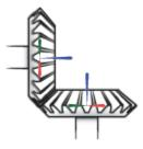
The block represents only the kinematic constraint characteristic to a bevel gear system. Gear inertia and geometry are solid properties that you must specify using Solid blocks. The gear constraint model is ideal. Backlash and gear losses due to Coulomb and viscous friction between teeth are ignored. You can, however, model viscous friction at joints by specifying damping coefficients in the joint blocks.
