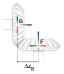
• The distance between the base and follower frame origins along the z-axis of the follower frame, denoted  $\Delta z_{\rm F}$ , must be equal to:
